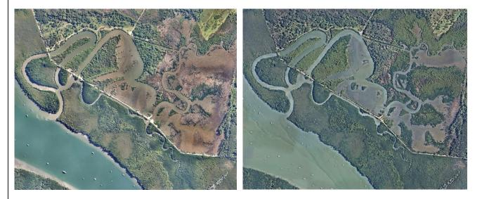
The picture above (left image) shows the bund walls surrounding the Trinity Inlet built for the production of sugar cane in 1970s that resulted in GHG emissions and acid sulfate soils. The reintroduction of tidal flow in 2000s resulted in the recovery of vegetation by 2021 (right image; source: Nearmap Australia Pty Ltd).
